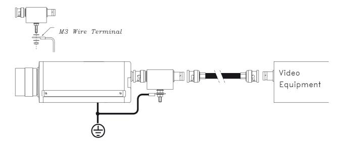
Monitor, matrix, multiplexer, videorecorder, etc. video IN protection only
